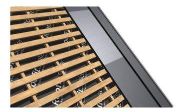
Install the next BIPV module on top with a 200 mm overlap to ensure adequate water resistance.
