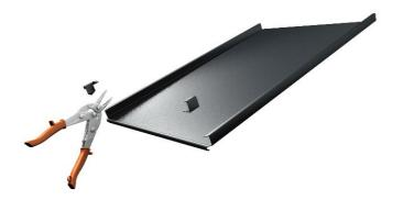
Step 1. The bottom part of the passive metal need prepared by cutting the seams and forming a backbend.
