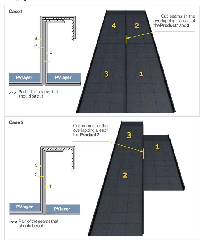
All modules have an overlap area of 200 mm for the purpose of waterproofing the joints. 3 mm gap is left between the lower and upper PV layer. Most PV modules require cuts in the overlap seams, which should be approximately 20 mm shorter than the intended overlap.
