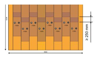
In the brick-pattern layout the next column of the BIPV modules is shifted up or down. The minimum recommended distance between 2 horizontal seams is 250 mm.
