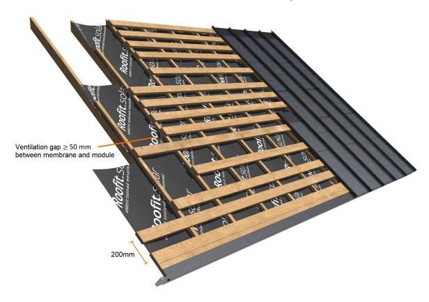
When installing the modules, pay attention to where the battens are placed in relation to the junction box. Each BIPV module has a junction box that needs to be placed between the battens. Ensure everything fits and works correctly, please consider **150 mm of free space** for the junction box, wires and any potential misplacements. If the battens are in the way of the junction box, move them up or down before installing the module.
