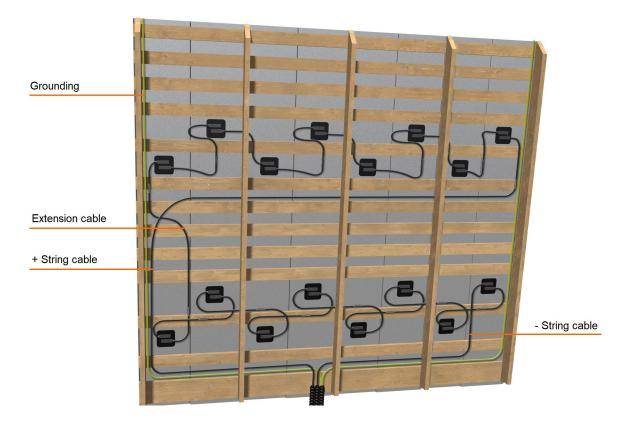
The inverter cables ([-] String, [+] String), the grounding and extension cables connecting BIPV modules should be positioned on site before the installation. Depending on local regulations, loose cables might be required to be fixed with cable insulation net.
