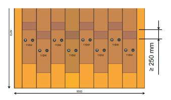
Step 10. In the brick-pattern layout the next column of the BIPV modules is shifted up or down. The minimum recommended distance between 2 horizontal seams is 250 mm.
