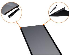
Step 1. The top part of the left and right seams must be cut in the same manner as already done for the BIPV modules in the length of 205mm before installing the next BIPV module on top.
