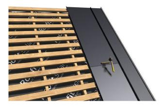
The backbend of the regular metal can be flattened with a wooden board and bumping mallet.
