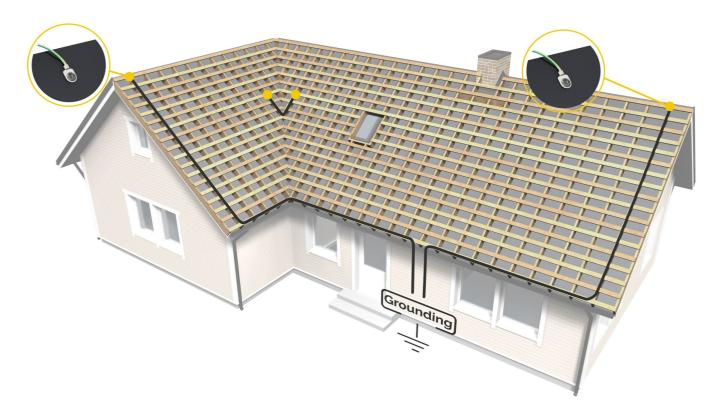
Each BIPV system must be connected to the grounding cable to ensure electrical safety. All Roofit.Solar modules that are seamed with each other are galvanically connected. Use adequate grounding cables with a cross-section of at least 4 mm<sup>2</sup> and A2 or A4 stainless steel screw. The grounding cable is connected to the uppermost metal sheet of the roof under the ridge cap. The grounding is finalized by connecting the grounding conductors to the equipotential grounding.
