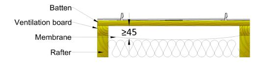
When installing the modules, pay attention to where the battens are placed in relation to the junction box. Each BIPV module has a junction box that needs to be placed between the battens. Consider **200 mm of free space** for the cable tray, junction box, wires and any potential misplacements. If the battens are in the way of the junction box, move them up or down before installing the module.
