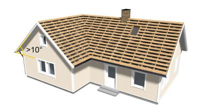
The use of an underlayer membrane under Roofit.Solar BIPV modules is mandatory. Any penetration (e.g. chimney, pipes etc.) to the roof must be adequately sealed to prevent leaks. The back of the module must be kept free of foreign objects that are not part of the support structure. The minimum allowed **ventilation gap of 45 mm** is required between the batten and the moisture barrier.
