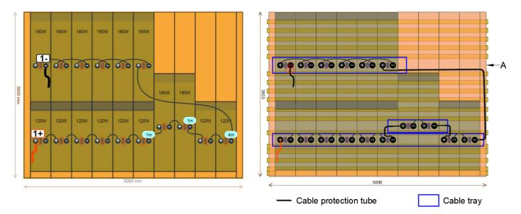
Cable trays, inverter cables ([–] String, [+] String), the grounding and extension cables should be positioned on site before the installation. Depending on local regulations, loose inverter and extension cables might be required to be placed in the cable protection tube. Back of the PV module and connectors must be placed inside the cable tray.
