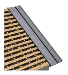
**Step 5.** While placing the next module on top, make sure to leave minimum 3 mm gap between two glasses.
