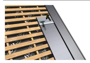
**Step 2.** The seams in the Roofit.Solar Products overlapping area should be cut.
