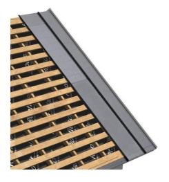
**Step 3.** Install the next PV module on top with a 200 mm overlap
