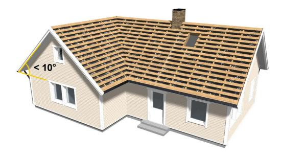
The minimum and maximum allowed center-to-center batten spacing is 200 and 400 mm respectively. Roofit. Solar best practices recommend using a spacing of 200 mm to ensure adequate cooling and wind uplift resistance. The minimum allowed ventilation gap between the batten and the moisture barrier is 45 mm, which can be achieved by using a ventilation board of appropriate thickness. A minimum of 200 mm from the bottom of the roof should be fully decked.
