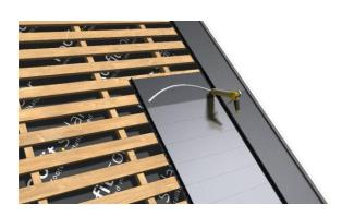
Step 4. Butyl sealant is applied in a curved line in the middle of the overlap section, leaving a few centimeters gap at the end for condensation water drainage.
