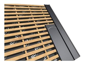
**Step 2.** Sound insulation band under the regular metal sheet helps to reduce wind noise and oil canning.
