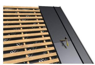
**Step 3.** The folded end of the metal sheet must be inserted under the extension flashing and then pulled toward the ridge to fix it into place. Backbend of the regular metal can be flattened with a wooden board and bumping mallet.
