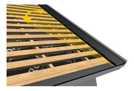
**Step 2.** First, fix the roofing sheet with just one fastening clip at the bottom corner of the sheet.
