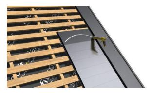
**Step 4.** Butyl sealant is applied in a curved line in the middle of the overlap section, leaving a few centimeters gap at the end for condensation water drainage.
