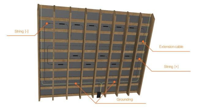
The inverter cables (String [–], String [+]), the grounding and extension cables connecting the Roofit.solar Products should be positioned on site (i.e. between battens) before the installation. Loose cables should be fixed to the wooden structure with the help of cable holder clips. In order for the PV system to maximize EMC (Electromagnetic compatibility) and to minimize the electromagnetic radiation, cabling should be positioned in a way to minimize the area of the wiring loop.
