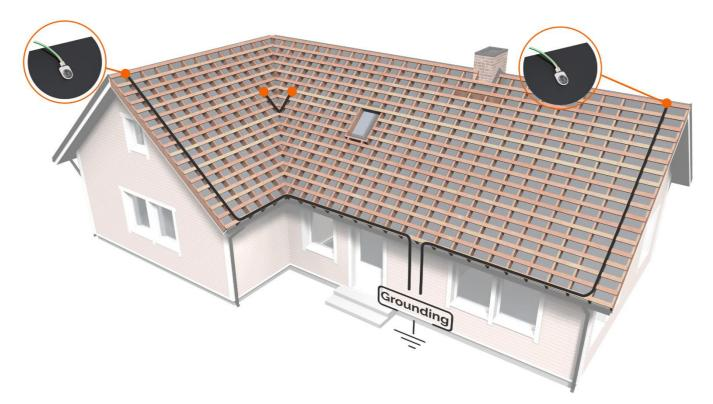
Each PV system must be connected to the grounding cable to ensure electrical safety. All Roofit.Solar products that are seamed with eachother are galvanically connected. Roofit.Solar recommends 2 grounding cables per roof, to provide the possibility to measure ground connection quality.
