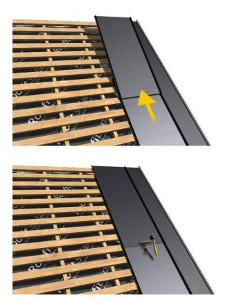
**Step 3.** The folded end of the metal sheet must be inserted under the extension flashing and then pulled toward the ridge to fix it into place. Backbend of the regular metal can be flattened with a wooden board and bumping mallet.
