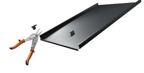
**Step 1.** Prepare the top metal part by cutting the seams and forming a backbend.
