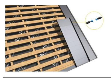
**Step 3.** Before fixing the PV module, cut the seams (if needed) andmake sure to connect the cable with the previous module/inverter cable. Remove the dust caps and push the connectors together until you hear a \*click\*. Bring the second cable of the PV-module out from the side to ease the connection of the next module afterwards.
