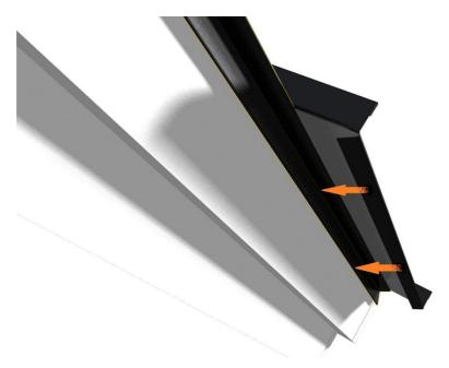
**Step 1.** The bottom sheet shall be installed as required in the Installation manual of the double seam metal with metal folding under the eave.
