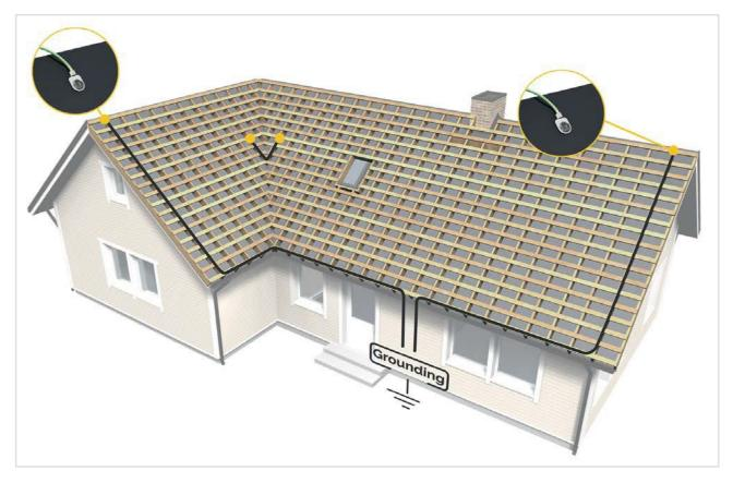
Each PV system must be connected to the grounding cable to ensure electrical safety. All **Roofit**.solar products that are clicked with each-other are galvanically connected. **Roofit**.solar recommends 2 grounding cables per roof, to provide the possibility to measure ground connection quality.
