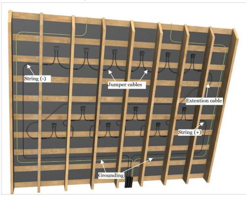
The inverter (String [-], String [+]), the grounding and extension cables connecting the Roofit.solar Productsshould be positioned on site (i.e. between battens) before the installation. Loose cables should be fixed to the wooden structure with the help of cable holder clips.
