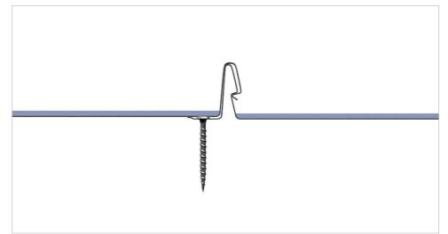
Pay attention to the fixing tightness and screwing direction. Screws fixed too tight will hinder the sheets' thermal expansion.
