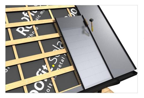
**Roofit**.solar module must be aligned with the edge of the previous module, which is already fixed to the roof, and locked in place using a bumping mallet proceeding from the eaves to the ridge. Make sure the bottom ends of the modules are in line.
