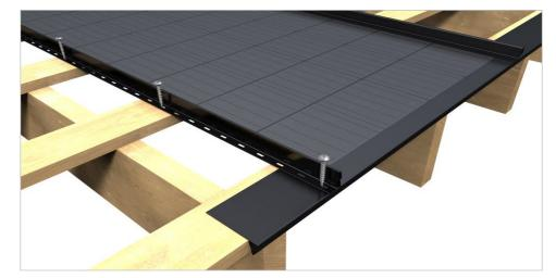
The screws should be positioned approximately in the middle of the holes.
