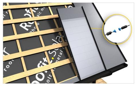
The PV cables with female and male connectors should be in accessible positions before fastening the **Roofit**.solar modules to the battens.
