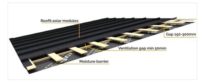
Special attention must be paid to the positioning of the battens in respect to the installation of the Product. Each Product has a junction box that must be placed in between of the battens to guarantee safe installation.
